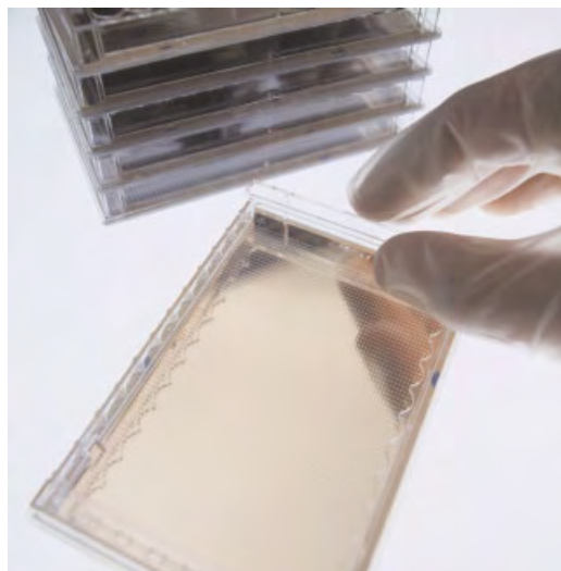
Fig. 9.5 Chemical microarrays as they are used at Graffinity. The array is based on a microtiter plate footprint and carries up to 10,000 individual compounds spotted in rows and columns onto an optical microstructure.
